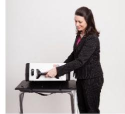
2. Stand at the front of the booth. Reach under the front of the booth top and push the latch away from you to secure the Touch Writer to the booth. ▶
