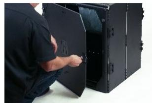
5. Follow local procedures to remove the tamper seal from the Verity Scan handle, if applicable. Unlock the case (if locked). Open the case and remove the power brick and power cord from the storage compartment. Close the compartment and case. ▶
