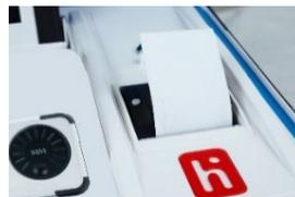
2. To open the paper compartment: While standing in front of the device, pull the lever on the top of the printer cover towards you and lift up to open the paper compartment. ▶
