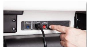
**IMPORTANT: Wait for the Verity Scan to be completely powered down and showing a black screen if you will be unlocking and removing the tablet. If stowing the tablet, make sure to lock it in place with the key and pull the blue latch down to secure it in place.**
