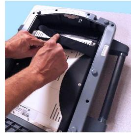
10. Insert one sheet of thermal paper. Once the paper has been fed into the printer, lay the sheet flat as shown.
