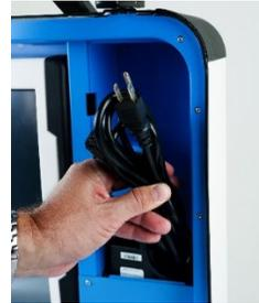
3. Plug the power cord into the power brick, and then plug the power brick into the back of the Verity Controller (flat side up). ▼
