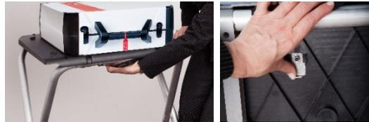
3. Follow local procedures to remove the tamper seal from the Verity Duo handle, if applicable. Unlock the case (if locked). Open the case and remove the power brick and power cord from the storage compartment. Close the compartment and case. ▶
