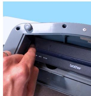
8. Connect the USB cable on the inside of the Duo Go carrier to the port on the side of the tablet. A tamper seal may be used to secure the cable; remove this seal first, if applicable.
