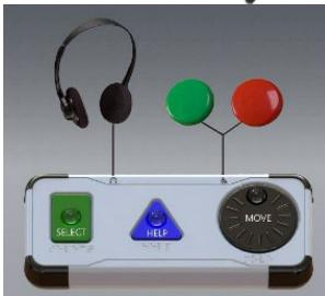
**Verity Touch Writer Duo** may be used with **Verity Access**, an Audio-Tactile Interface (ATI) intended for voters that cannot, or prefer not to, use the touchscreen. Verity Access includes two connection ports: the left connection port for headphones, and the right connection port for any dual-switch input device (such as tactile switches or sip-and-puff devices). For more information, see page 27.
