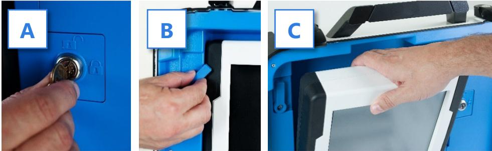
9. Seat the tablet in the cradle (A), tilt it back (B), and lock it in place (C). ▼
