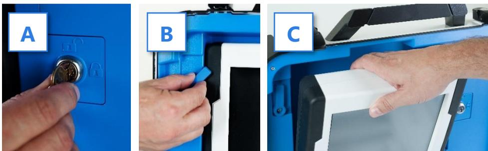
9. Seat the tablet in the cradle (A), tilt it back (B), and lock it in place (C). ▼
