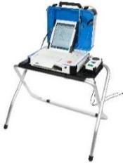
With **Verity Touch Writer Duo Standalone**, poll workers activate a ballot and voters mark and print a paper vote record. The voter will then scan their printed vote record using a Verity Scan device or deposit the printed record into a secure ballot box to be scanned centrally.
