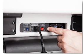
**NOTE:** The Verity power cord has a locking connector. When inserting the connector into a Verity device, it will make a small “click.” To disconnect the power cord, grasp the cord at the base of the black connector molding where it connects to the Verity device, and slide back the sleeve. This will unlock the connection so that the cord may be removed.
