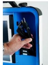
4. Plug the power cord into the power brick, and then plug the power brick into the back of the Verity Duo (flat side up). ▼
