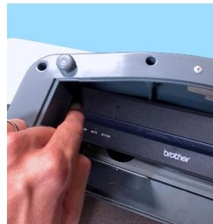
7. Connect the USB cable on the inside of the Duo Go carrier to the port on the side of the tablet. A tamper seal may be used to secure the cable; remove this seal first, if applicable.
