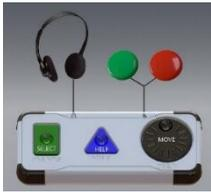
Verity Duo may be used with **Verity Access**, an Audio-Tactile Interface (ATI) intended for voters that cannot, or prefer not to, use the touchscreen. Verity Access may be used with headphones and with any dual-switch input device (such as tactile switches or sip-and-puff devices). For more information, see page 19.
