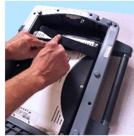
9. Insert one sheet of thermal paper. Once the paper has been fed into the printer, lay the sheet flat as shown.
