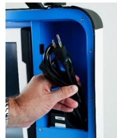
6. Plug the power cord into the power brick, and then plug the power brick into the back of the Verity Scan (flat side up). ▼
