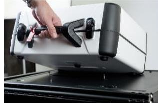
3. Reach inside the ballot box and pull the cord down and away from you to lock the lid and the Verity Scan in place. ▶
