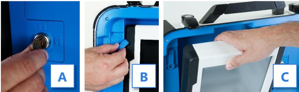
7. Seat the tablet in the cradle (A), tilt it back (B), and lock it in place (C). ▼
