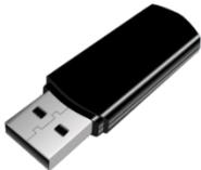
**vDrives** are used to transfer digital ballot styles from the Verity election definition software to Verity Print, and to transfer device audit log data from Verity Print to Verity software (vote data is not stored on Verity Print). vDrives are inserted into a standard USB port located in a locked and sealed compartment; each Verity Print has its own vDrive.
