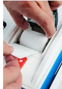
4. Close the printer cover. The paper must extend out from underneath the front edge of the cover. The white button can be used to advance the paper. ▶
