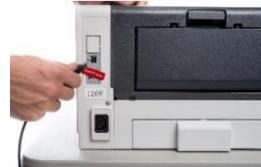
3. Insert the printer power cord into the printer and the other end into an outlet or UPS/battery backup. ▶
