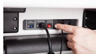
12. (*if applicable*) If your jurisdiction uses the AutoBallot barcode reader: Wait until the Verity Print finishes powering up and displays the **Enter Poll Worker Code** screen, and then connect the AutoBallot barcode reader to the USB connection located on the vDrive compartment above the report printer. ▶
