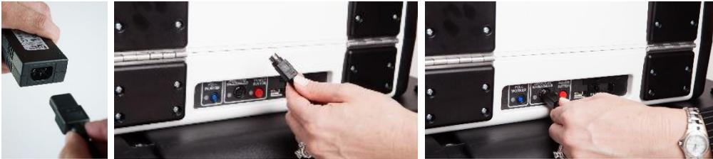
4. Plug the flat end of the USB printer cable from the ballot printer into the back of the Verity Print, with the notch facing up. ▼
