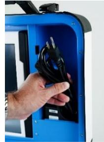
3. Plug the power cord into the power brick, and then plug the power brick into the back of the Verity Print (flat side up). ▼
