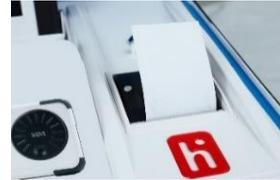
2. To open the paper compartment: While standing in front of the device, pull the lever on the top of the printer cover towards you and lift up to open the paper compartment. ▶
