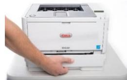
b) Load paper in the tray. If necessary, push the blue tab and pull the paper guide to the appropriate setting (Letter/8.5"x11", or Legal/8.5"x14"). Paper sizes larger than 8.5"x14" require a tray extender (not available in all jurisdictions). ▶
