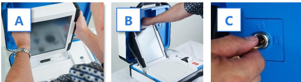
8. Verify the Verity Print device seals, per local procedure.
