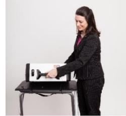
2. Stand at the front of the booth. Reach under the front of the booth top and push the latch away from you to secure the Touch device to the booth. ►
