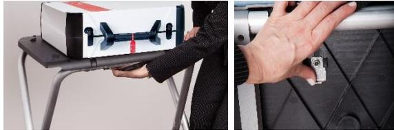
3. Follow local procedures to remove the tamper seal from the Verity Touch handle, if applicable. Unlock the case (if locked). Open the case and remove the power brick and power cord from the storage compartment. Close the compartment and case. ►
