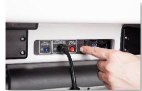
**IMPORTANT: Wait for the Verity device to be completely powered down and showing a black screen if you will be unlocking and removing the tablet. If stowing the tablet, make sure to lock it in with the key *and* pull the blue latch down to secure it in place.**
