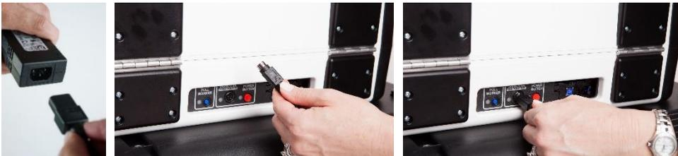
5. Insert a booth connection cord into one of the available ports on the back of *Verity Touch*. Insert the other end of the cord into one of the available ports on the back of the *Verity Controller*. ▶
