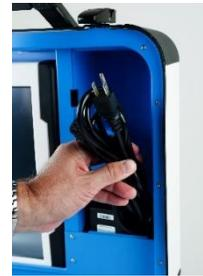
4. Plug the power cord into the power brick, and then plug the power brick into the back of the Verity Touch (flat side up). ▼
