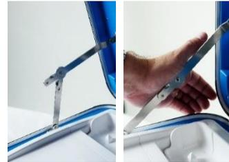
7. Unlock (A), unlatch (B) and remove (C) the tablet. ▼
