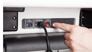
12. During the power on process, the Verity Touch screen will display a Power-On Self Test report. Any hardware or connection issues will be highlighted in yellow; if any issues are noted, check connections and restart the device using the red power button on the back of the device.
