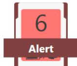
**Alert:** There is an error or issue with this Touch device; Go to the Touch voting booth and follow the directions on the screen. If the battery is low, reconnect the Touch device to AC power.
