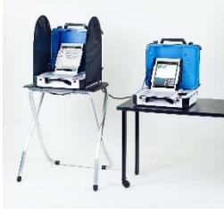
**Verity Controller** and **Verity Touch** make up the Verity Direct Record Electronic (DRE) voting system. Poll workers issue Access Codes with Verity Controller, which voters use to access, mark and cast digital ballots via a touchscreen on a Verity Touch device. Multiple Verity Touch devices can be connected to a single Verity Controller device.
