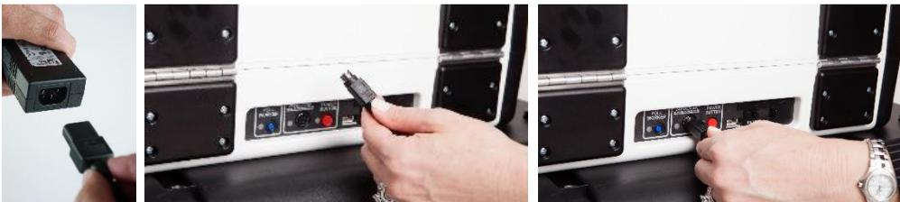
5. Plug the flat end of the USB printer cable from the ballot printer into the back of the Verity Touch Writer, with the notch facing up. ▼
