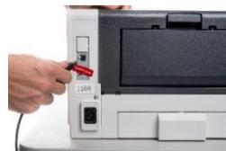
3. Insert the printer power cord into the printer and the other end into an outlet or UPS/battery backup. ▶
