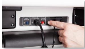
**NOTE:** *The Verity power cord has a locking connector. When inserting the connector into a Verity device, it will make a small “click.” To disconnect the power cord, grasp the cord at the base of the black connector molding where it connects to the Verity device, and slide back the sleeve. This will unlock the connection so that the cord may be removed.*
