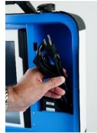
4. Plug the power cord into the power brick, and then plug the power brick into the back of the Verity Touch Writer (flat side up). ▼
