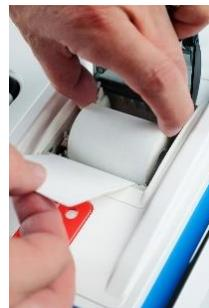
4. Close the printer cover. The paper must extend out from underneath the front edge of the cover. The white button can be used to advance the paper. ▶
