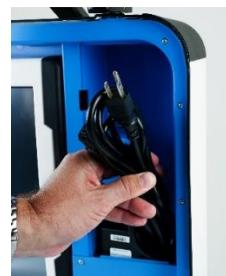
6. Plug the power cord into the power brick, and then plug the power brick into the back of the Verity Scan (flat side up). ▼
