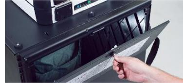
The emergency ballot slot on the top of the ballot box also feeds into this bag. This slot should remain sealed unless the Verity Scan device cannot accept ballots. ▶
