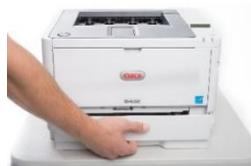
b) Load paper in the tray. If necessary, push the blue tab and pull the paper guide to the appropriate setting (Letter/8.5"x11", or Legal/8.5"x14"). Paper sizes larger than 8.5"x14" require a tray extender (not available in all jurisdictions). ▶
