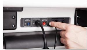
**IMPORTANT: Wait for the Verity Touch Writer to be completely powered down and showing a black screen if you will be unlocking and removing the tablet. If stowing the tablet, make sure to lock it in with the key *and* pull the blue latch down to secure it in place.**
