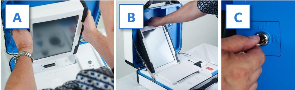
10. Verify the Verity Scan device seals, per local procedure. Attach privacy screens to each side of the ballot box, if applicable. ►
