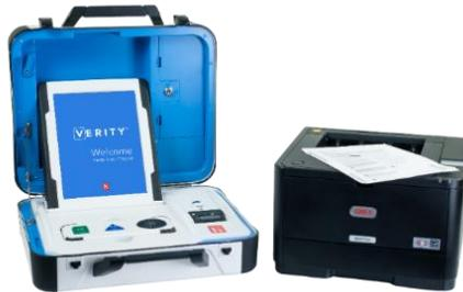
**Verity Access** is an Audio-Tactile Interface (ATI) intended for voters that cannot, or prefer not to, use the touchscreen. Verity Access includes two connection ports: the left connection port for headphones, and the right connection port for any dual-switch input device (such as tactile switches or sip-and-puff devices).
