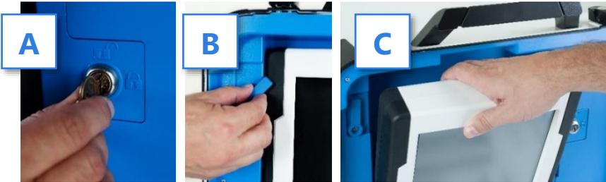
6. Seat the tablet in the cradle (A), tilt it back (B), and lock it in place (C). ▼
