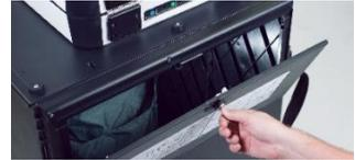
The emergency ballot slot on the top of the ballot box also feeds into this bag. This slot should remain sealed unless the Verity Scan device cannot accept printed vote records. ▶
