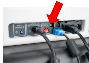
13. During the power on process, the Verity Duo screen will display a Power-On Self Test report. Any hardware or connection issues will be highlighted in yellow; if any issues are noted, check connections and restart the device using the red power button on the back of the device. ►
